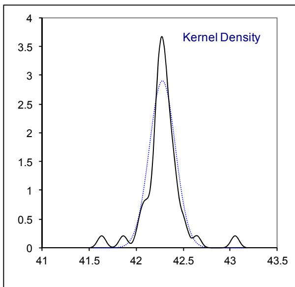
Determination of Kinematic Viscosity at 100°C on sample #15220; results in mm/s<sup>2</sup>.
