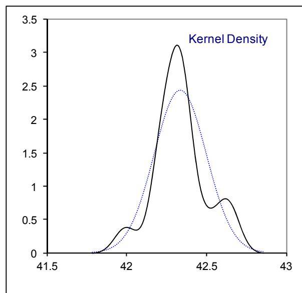
Determination of Viscosity Stabinger at 100°C on sample #15220; results in mm/s<sup>2</sup>.
