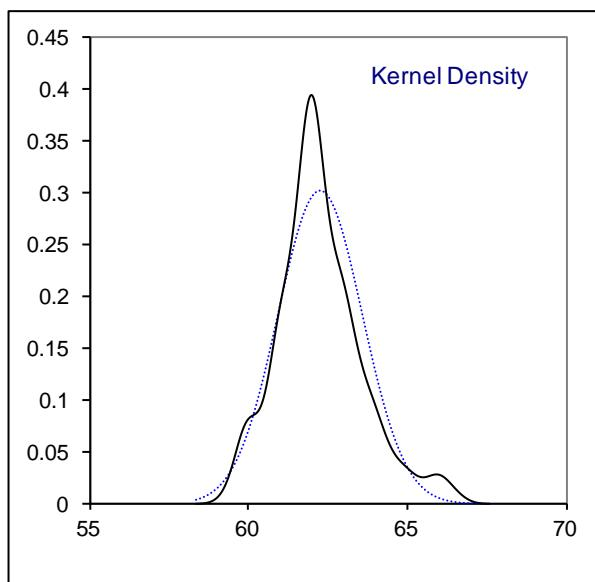
Determination of Kinematic Viscosity at 40°C on sample #16025; result in mm<sup>2</sup>/s
