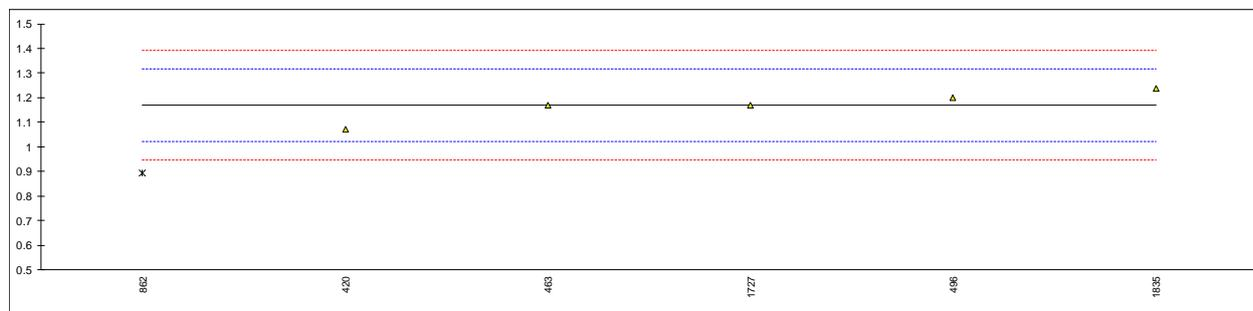
Determination of Existent Gum (solvent washed) on sample #18083; results in mg/100ml
